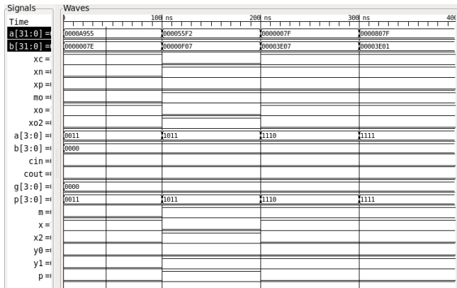
Fig. 5: Verilog simulation of Booth multiplier stages
